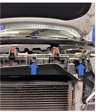
9. Undo the 10mm bolt securing the lower air feed and then pull it towards the front of the car to allow the upper radiator air guides to be removed.
