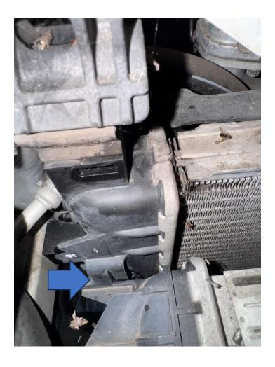
12. Reinstall the air-con radiator onto the mountings on the radiator that used to hold the intercooler.
