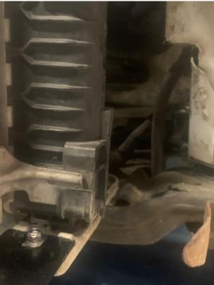
19. Install the centre bracket onto the intercooler using the supplied M6 fixings and then hang the intercooler on the crash bar. Use the supplied M4 bolts with Nyloc nuts with washers to go through the existing holes in the crash bar and tighten to secure, as shown.
