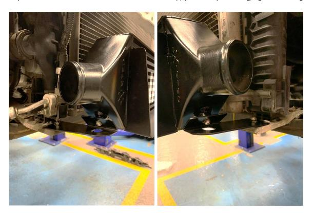
21. Remove the O-ring from the original pipe removed in Step 16 and install onto your new AIRTEC Motorsport pipe. Then fit it onto the car using the supplied M6 fixings.
