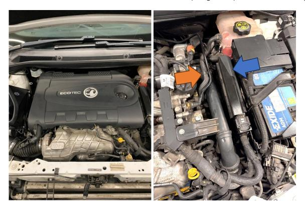
17. Remove the 10mm bolt holding the boost pipe bracket in place, followed by the three T27 Torx bolts holding the flange onto the throttle body. The pipe can then be lifted up and rotated until it comes out, but take care not to get it caught up with any wiring or hoses.
