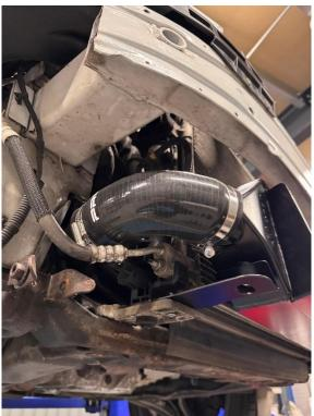
24. Ensure all fixings and clips are tight and then all parts can be reinstalled in reverse of removal - except for the two side air guides removed in Step 7. The left-hand side guide cannot be reinstalled and the right-hand side guide needs to be cut, as shown, before it can be reinstalled.
