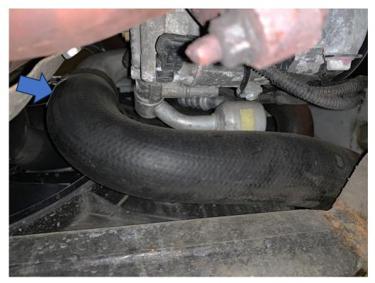
15. Undo the two 13mm bolts holding the upper section of the radiator in place. This will allow you enough room to rotate the boost pipe out in later steps.
