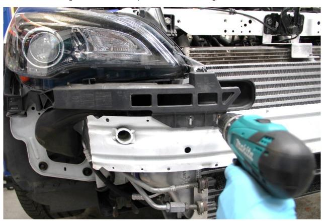
11. Remove the two bolts under each headlight. Then lift the headlight upwards to carefully release it. To prevent damage to the headlights, store them in a safe place away from the working area.
