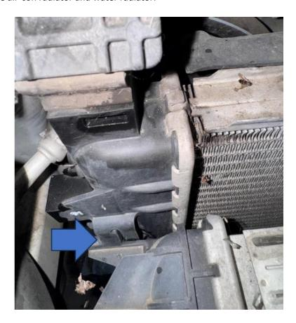
15. Reinstall the air-con radiator onto the mountings on the radiator that used to hold the intercooler.
