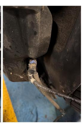
6. Remove the plastic air guides both sides by unclipping them and rotate them free.
