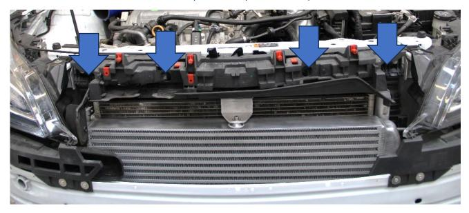
8. Remove the three nuts securing the power steering cooler and hang from it from the crash bar using a strong cable tie. **Please note:** this is not a standard intercooler shown.
