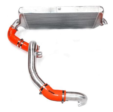
21. Start fitting this side by removing the rubber seal from the original turbo outlet pipe removed in Step 19 and carefully insert it into your new AIRTEC Motorsport turbo outlet pipe. Then fit the outlet pipe using the two supplied M6x16mm Socket Head bolts provided. **Do not fully tighten yet to allow movement.**
