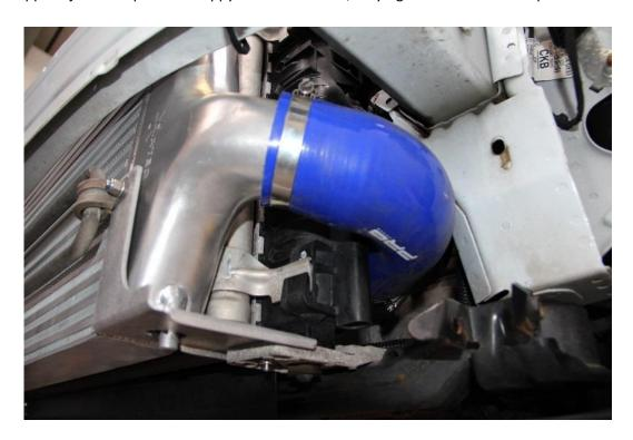
23. For the cold side of the pipework going from the throttle body to the intercooler, please make note of the picture for reference.
