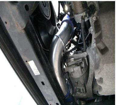
25. Finally, check all hose clamps and fixings are correctly tightend and in the correct position. You can then refit the headlights by riveting them back onto the crash bar and then refit the bumper in reverse of removal.
