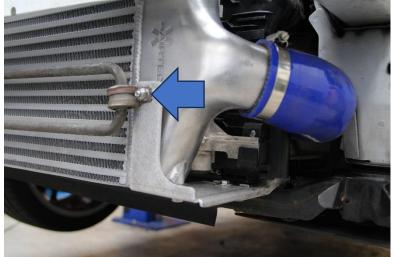
9. Remove the two bolts securing the power steering cooler brackets.
