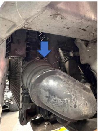
13. Follow each boost hose up and loosen the jubilee clips securing it in place, as highlighted below in the picture of it removed. You can then remove both pipes from the car.
