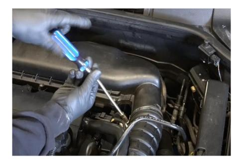
2 Now remove the four T20 Torx bolts from the lid of the air box and remove the lid and original air filter.
