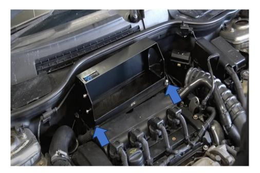
4. Insert the AIRTEC Motorsport air filter into the air box and then install the filter adapter onto the side of the air box but don't bolt it in place yet. You will also need to insert the alloy pipe connector into the original pipework, as shown.
