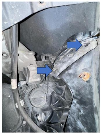
3. Under the car, undo the three Allen Key bolts attaching the undertray to the metal skid plate.
