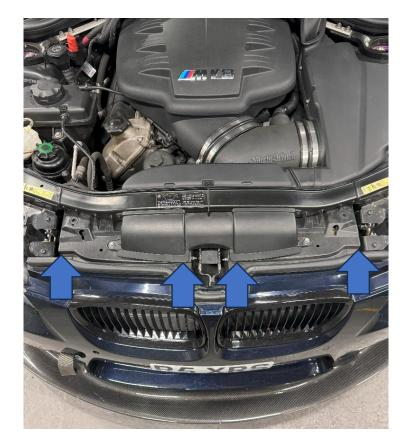
5. With the help of a second person, pull the edge of the bumper away until it releases. If your car is fitted with front parking sensors, then unclip the connectors before removing the bumper.
