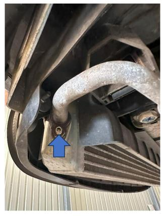
7. Remove the two T45 Torx bolts on the left-hand side and one T45 bolt on the right-hand side holding the c cooler in place. You can then slide it to the right-hand side and lower the left-hand side down to remove.
