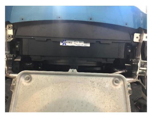
6. Finally, once in position, secure the intercooler in place reusing the original bolts and then reattach the original boost pipes using the same spring clips. You can then refit the undertray in reverse of removal.
