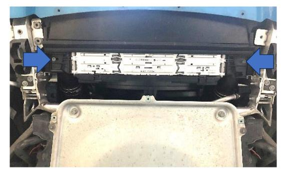
4. Carefully pull the plastic air guide down and then tilt the intercooler towards the front of the car to remove.
