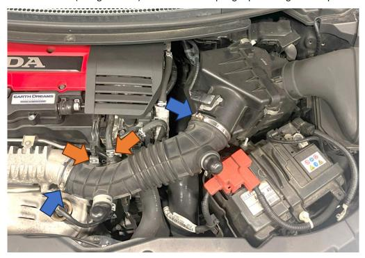
2. Now unclip the MAF sensor wiring connector and cable clip from the air box.
