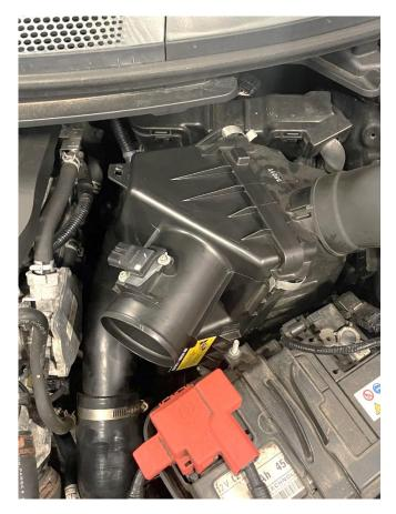
6. Finally, install the new Pro Hoses induction pipe and reconnect the MAF sensor and cable. Secure with the supplied jubilee clips and reconnect the take-offs removed in Step 1 with the smaller supplied jubilee clips.
