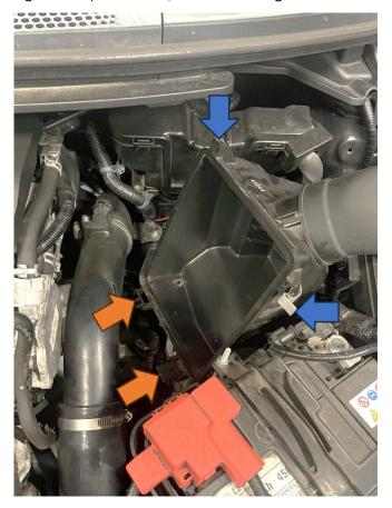
4. Install the AIRTEC Motorsport panel filter into the air box.
