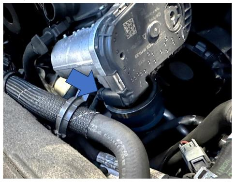
8. With the manifold removed you can now undo the four 8mm bolts holding the throttle body to the manifold and reinstall it, along with the throttle body gasket, onto the AIRTEC Motorsport manifold using the supplied M6x35mm flanged bolts.
