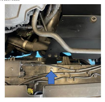
10. Secure the left-hand side of the new air box in place using four of the supplied push fits to hold it in place.
