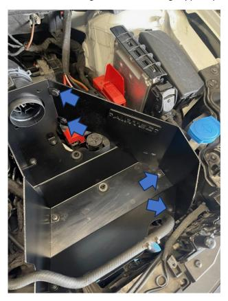
12. Bolt the MAF sensor housing to the new air box using the two supplied Button Head bolts with Nyloc nuts and washers both sides.
