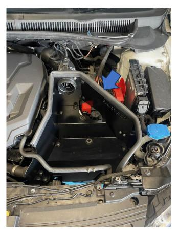
15. Place the vacuum line disconnected in Step 5 through the hole in the side of the air box and connect to the take-off on the bottom of the new induction hose. Then fit the hose to the MAF housing with the supplied jubilee clip, as shown, but do not fully tighten yet to allow adjustment.
