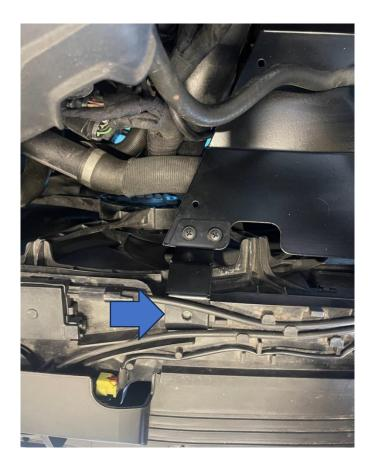
8. Use the hole in the bracket to make a mark and then drill a 7mm hole.
