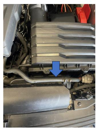
4. Undo the T27 Torx bolt on each side of the air feed and remove it from the car.
