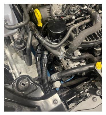
26. Use the supplied cable ties to secure the lines together at intervals.
