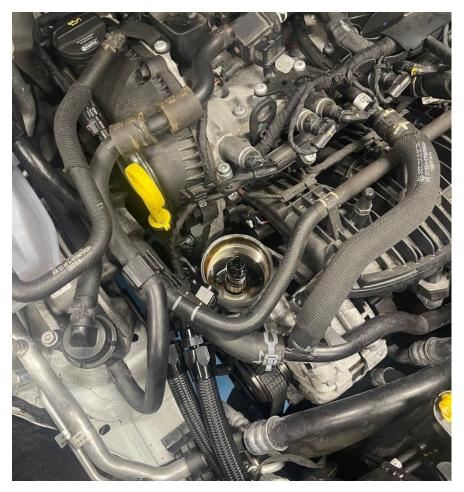
20. Now fit the supplied oil fitting adapter and tighten using a 27mm deep socket.
