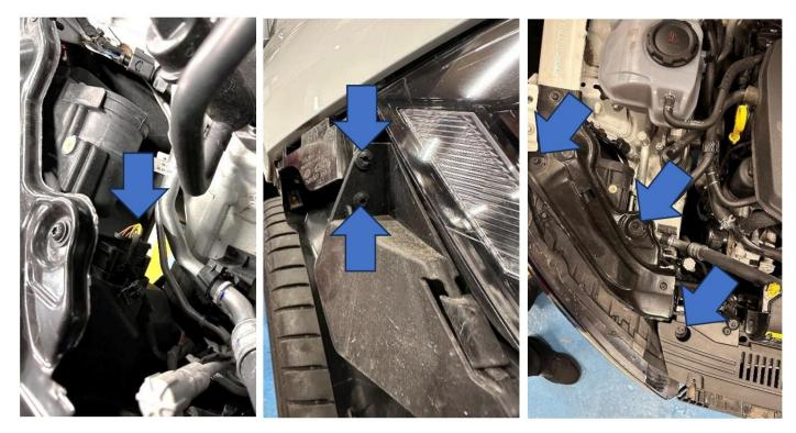
6. Remove the upper front plastic bumper support by undoing the two T25 bolts on top followed by the T27 bolt located each side and unclip the wiring harness as you remove the surround.
