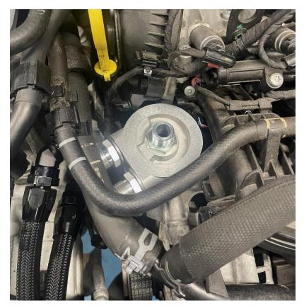
24. Attach both the oil lines in positon (they can go on either take off) and fully tighten them using a hose fitting spanner or adjustable spanner.
