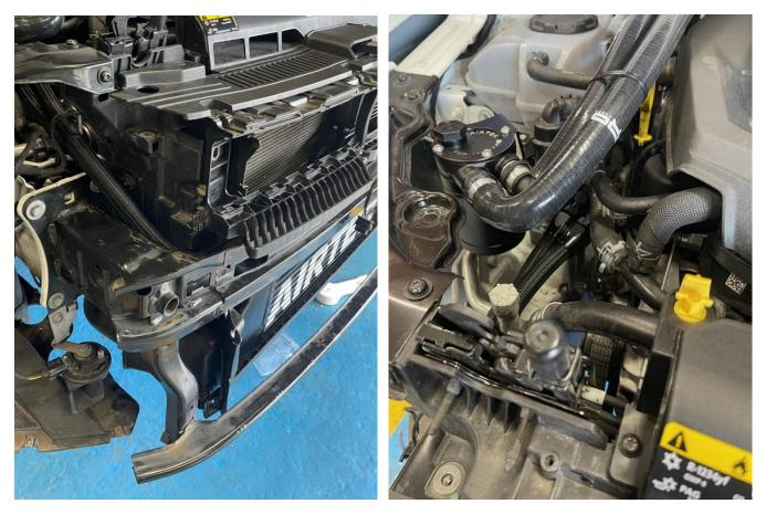
16. Bolt the right-hand side oil cooler bracket with the supplied M6x35mm Socket Head bolt and supplied alloy spacer between the bracket and plastic trim. On the left-hand side, reuse the original bolt removed in Step 6.
