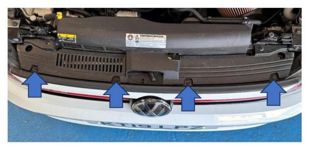
4. With the help of a second person, pull the corner of the bumper out each side. As the bumper comes forward you will need to disconnect a wiring plug on the left-hand side followed by two wiring plugs on the right-hand side and single plug in the middle behind the badge.
