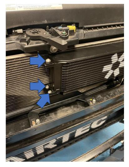
13. Attach the right-hand side bracket to the oil cooler using the remaining two M6 Button Head bolts with Nyloc nuts and washers. This will pass through the slot created in Step 8C. Fully tighten all bracket bolts now.
