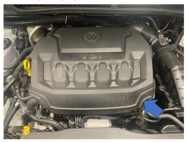
18. Locate the oil filter housing on the left-hand side of the engine.
