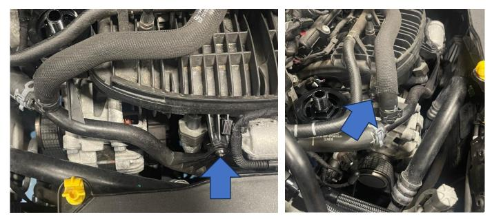
22. Once it is free, lift the pipework up to fit the supplied sandwich plate in place.
