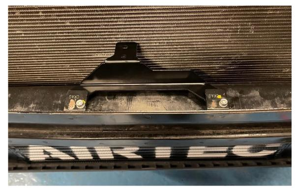
9. Fit the bottom bracket using the supplied M5 Socket Head bolts with Nyloc nuts and washers to secure it in place, but do not fully tighten yet to allow adjustment.
