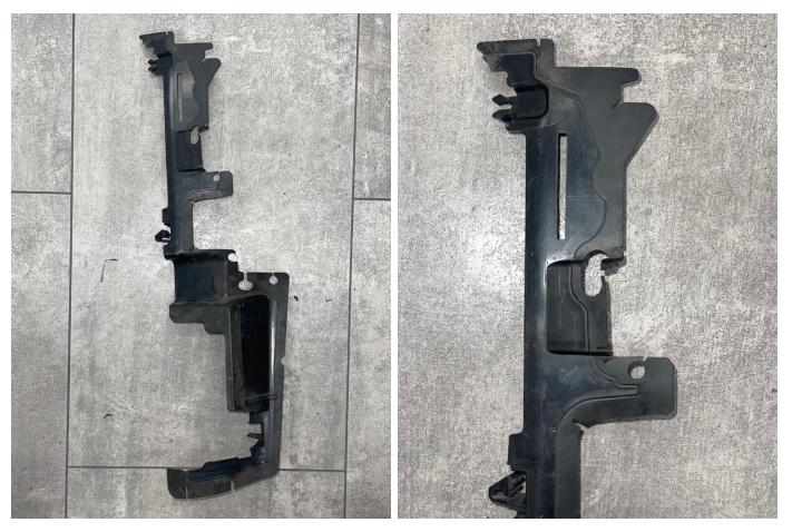
Once all the trimming is complete, refit the air guides onto the car.
