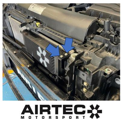
14. Hook the upper front plastic bumper support removed in Step 6 over the right-hand side bracket but do not bolt it up yet. Push the oil lines down between the crash bar and radiator surround, as shown.
