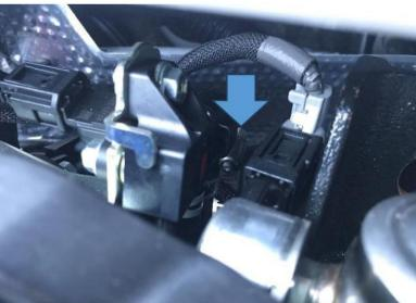
4. Locate the two 12mm bolts holding the inlet pipe in place. One bolt is easy to see at the top but the other is located out of sight underneath, so you need to locate it by hand. Then remove the wiring clipped to it using a trim removal tool and remove the pipe from the car.
