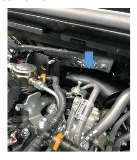
6. Undo the air box lid by unclipping the two clamps at the front and lift the lid. Remove the original panel filter and replace with the supplied AIRTEC Motorsport panel filter and then reattach the lid.
