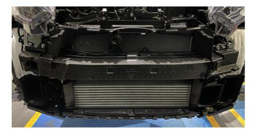
7. Remove the lower plastic trim by removing the three plastic clips using a trim removal tool.
