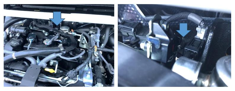
9. Undo the two 12mm bolts holding the inlet pipe in place. One bolt is easy to see at the top but the other is located out of sight underneath, so you need to locate it by hand. Then remove the wiring clipped to it using a trim removal tool and remove the pipe from the car.
