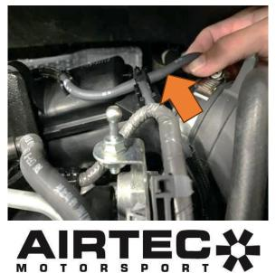
3 Unplug the MAF sensor and unclip the wiring harness from the top of the air box.
