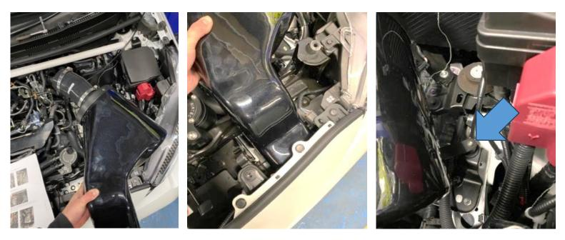
15. Now reinstall the MAF sensor into the new housing using the supplied M4x8mm Button Head bolts and once happy with the fitment and alignment of everything, fully tighten all jubilee clips.
