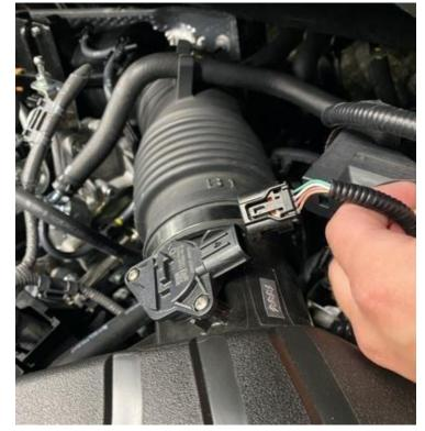
5. Using a trim removal tool, release the two trim clips that secure the air guide to the slam panel and then carefully remove the guide and put it aside.
