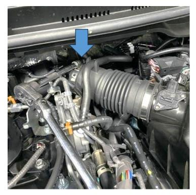
7. Now firmly but carefully pull the air box up and to the left so that you can access the wiring loom for the solenoid. Use a trim removal tool to gently unclip the wiring loom and then fully remove the air box from the car. Tuck the solenoid wiring up on the right-hand side and secure using a cable tie or similar.
