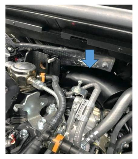
11. Install the smaller of the two supplied silicone connectors onto the intake pipe with the supplied jubilee clips. Do not fully tighten the jubilee clips yet to allow for adjustment
