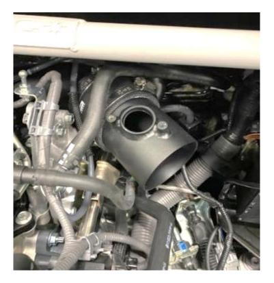
13. Before installing the air feed, you will need to stick the supplied foam strip in place to stop the intake's finish from being damaged, as highlighted below.
