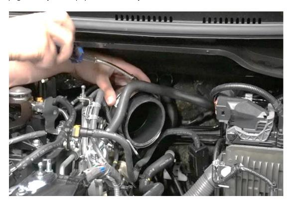
12. Slide your new MAF sensor housing pipe into the silicone hose and secure with a supplied M6 bolt and washer (blue arrow) to attach to the bracket. Then slide the second silicone hose with the supplied jubilee clips but do not fully tighten the jubilee clips yet to allow for adjustment.
