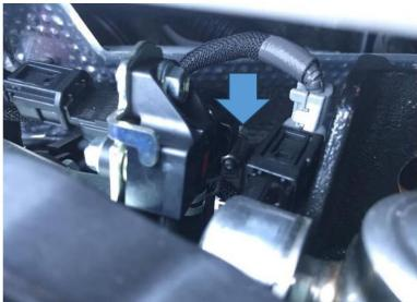
8. Undo the two 12mm bolts holding the inlet pipe in place. One bolt is easy to see at the top but the other is located out of sight underneath, so you need to locate it by hand. Then remove the wiring clipped to it using a trim removal tool and remove the pipe from the car.
