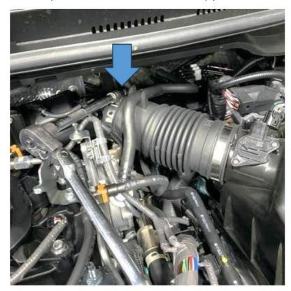
6. Now firmly but carefully pull the air box up and to the left so that you can access the wiring loom for the solenoid. Use a trim removal tool to gently unclip the wiring loom and then fully remove the air box from the car. Tuck the solenoid wiring up on the right-hand side and secure using a cable tie or similar.
