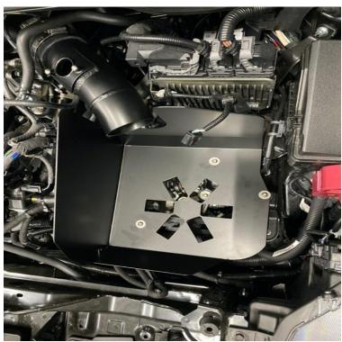
14. Now install the air filter. Position the filter to ensure there is no rubbing against the shield. Once happy with positioning of all parts, proceed to fully tighten all jubilee clips.
