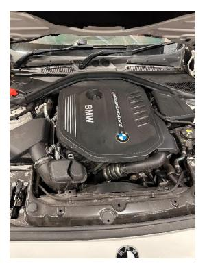
2. Unplug the MAF sensor and undo the jubilee clip. The air box can then be removed by firmly but carefully pulling it up at the corners to release it from its rubber mounts.
