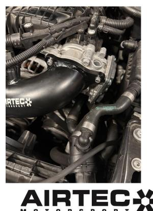
15. Finally, reconnect the MAP and temperature sensors, tighten the jubilee clips on the silicone hoses and fit the meth bung and tighten. The original parts can then be reinstalled in the reverse order of removal.
