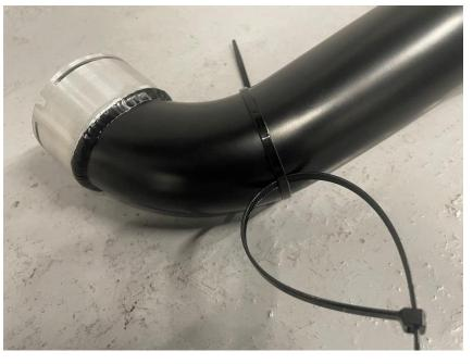
14. Place the second supplied jubilee clip onto the silicone hose and then install the upper part of the boost pipe and using the supplied M6 bolts and washers, tighten onto the throttle body. The weld around the flange can mean that the washer will start to deform as you tighten the top left bolt however this is perfectly fine.
