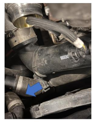
10. You can now remove the spring clip holding the pipe to the turbo. You will need to lift both edges so the clip sits in the groove, as shown. Then lift the centre of the clip to pull it away from the turbo and remove the pipe from the car.
