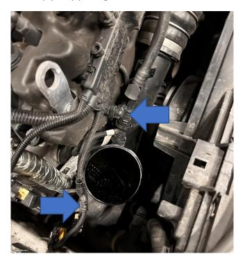
6. You will need to remove the spring clip highlighted. Use a flat-bladed screwdriver or similar to lift up the centre of the clip and then pull it upwards to release it. Once it is removed you can then pull the turbo elbow off.
