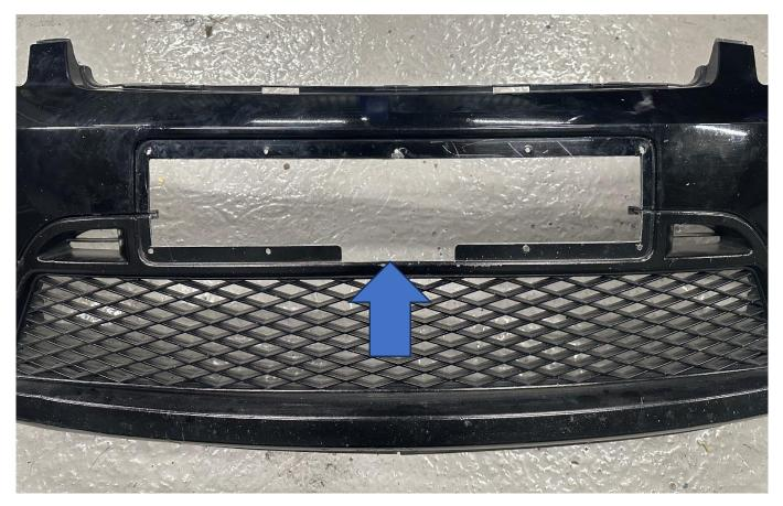
6. Finally, use the supplied nuts, bolts and washers behind to fit the air vent panel. You can then refit the bumper and/or grille in reverse of removal.
