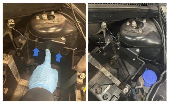
6. If your car is fitted with an aftermarket induction kit as seen here, it's best to remove it in order to allow extra room to run the hoses. If your car still has the original intake air box, you only need to remove the front air feed.
