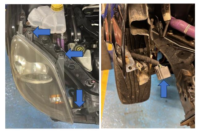
To remove the original power steering tank, undo the top bolt (blue arrow) and the two underneath (shown in second picture when removed). Then use a hose clamp tool to remove the return feed (orange arrow).
