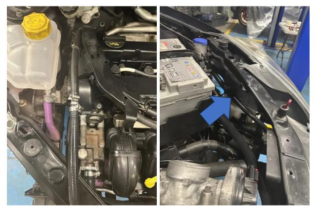
9. Fit the large hose to the bottom of the supplied expansion tank and secure with a provided jubilee clip. Then fit the smaller hose and attach it the tank's take-off and secure with a supplied jubilee, as shown.
