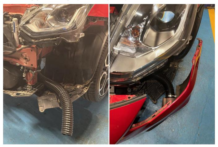
12. Finally, refit the boost hose removed in Step 7 and then the bumper in reverse of removal.
