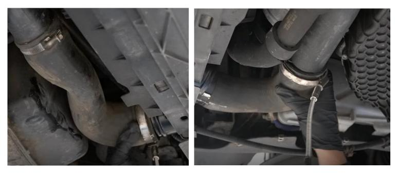
2. Remove the cold side pipe work by loosening the two T27 Torx bolts securing it in place. You will also need to unplug the sensor, which is located on the pipework.
