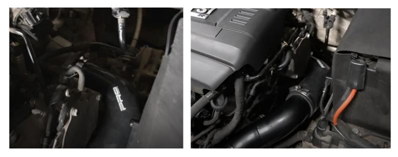
12. Now the hot side pipework is roughly in place you can install the silicone hose which goes from the alloy pipework to the intercooler.
