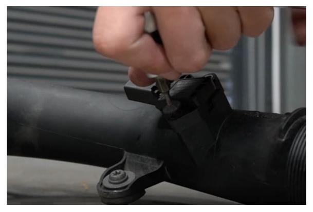
8. Install the silicone hose onto the throttle body and secure the jubilee clip using a hose clamp driver.
