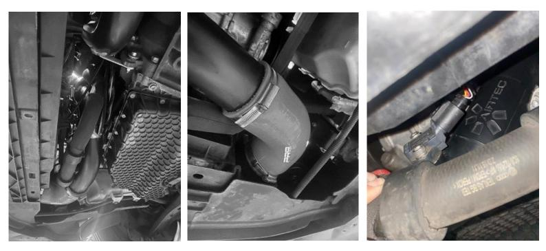
10. You can now install the bracket onto the threaded boss using the supplied M6x12mm bolt and M6 Mudguard washer. Once in place, it can be lined up with the thread already located in the engine block and secured using the supplied M6x16mm Socket Head bolt and washer.
