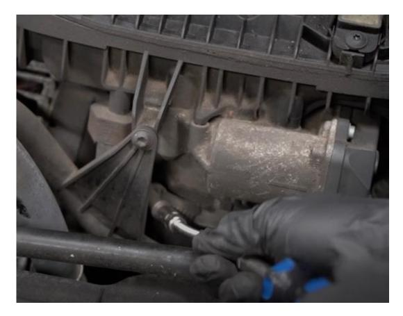
4. Remove the T27 Torx bolts securing the hot side boost pipe in place.
