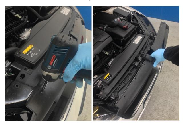
2. This gives access to three T30 Torx bolts that hold the bumper to the crash bar; remove these.
