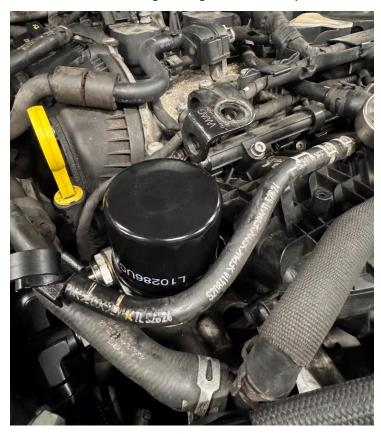
18. Install the supplied bracket to position the coolant hose out of the way. Reuse the original Torx bolt fitting at the bottom and the supplied M5 fixings to secure the hose to the bracket.
