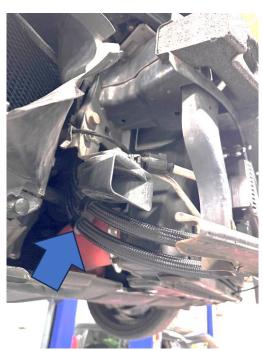
16. Install the oil lines onto the sandwich plate. Rotate it so that it has sufficient clearance and then tighten the centre bolt to secure it in place.
