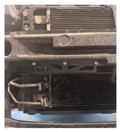
8. Install the oil cooler onto the bracket using the supplied M6x14mm bolts, washers and Nyloc nuts. Install the supplied O-rings between the oil cooler and bracket to reduce the vibration.
