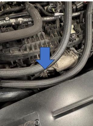
14. Once it is free, lift the pipework up and fit the supplied sandwich plate with centre bolt as shown, but do not fully tighten yet.
