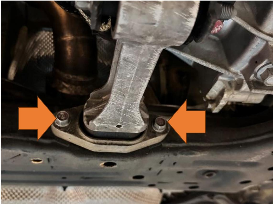
4. Install the new base onto the body of the vehicle noting the orientation as per the picture using the supplied M10 bolts.
