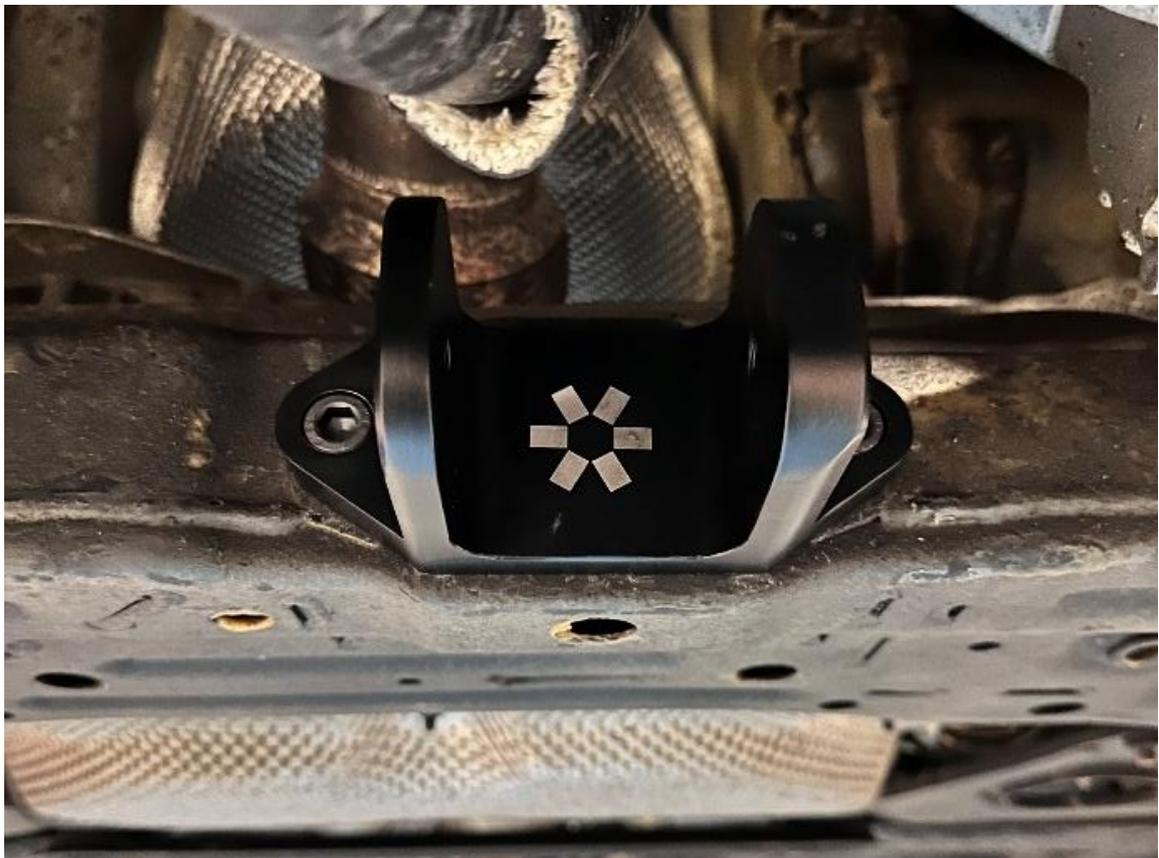
5. Install the torque mount body onto the base using the supplied M12 bolt, noting the orientation from the picture below.
