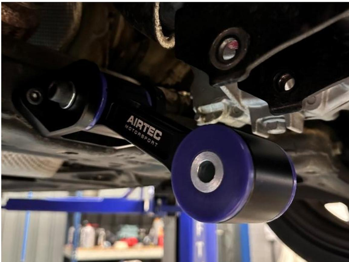
6. Finally, re-install the original 17mm bolt removed in Step 3, making sure to install the supplied spacer between the bush and the bracket.
