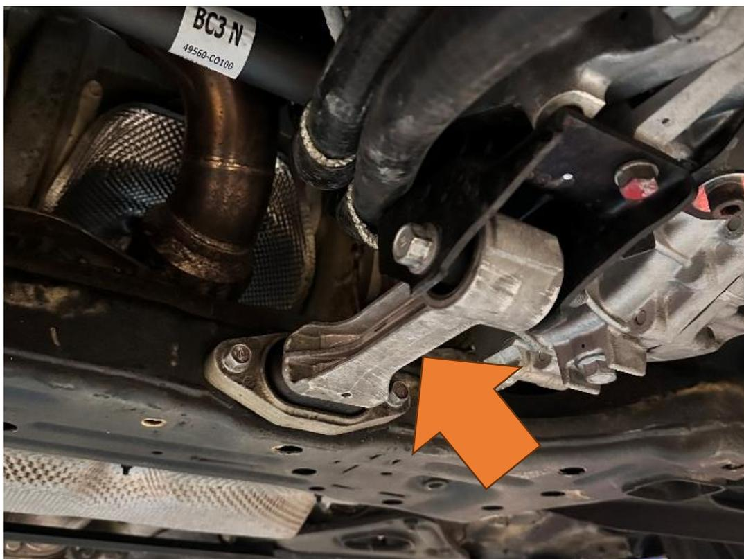
2. Undo the 17mm bolt holding the torque mount to the bracket.
