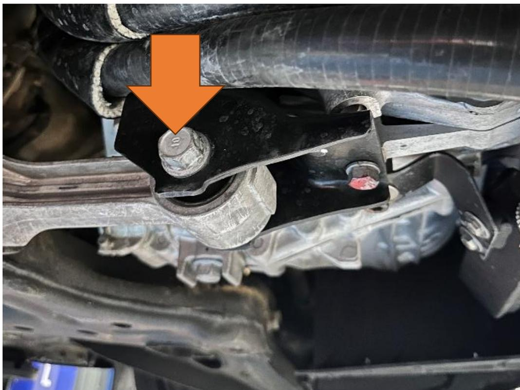
3. Undo the two 14mm bolts holding the torque mount base to the body of the car.
